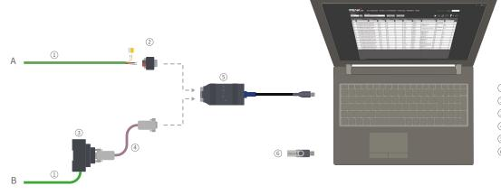
① KNX bus ② KNX-WAGO adapter ③ DIN rail adapter ④ Extension cable
