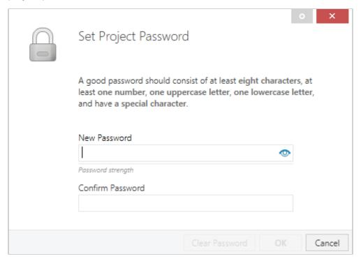
This password protects the ETS project from unauthorized access. This password is not a key that is used for KNX communication. The entry of the password can be bypassed with "Cancel", but this is not recommended for security reasons.
