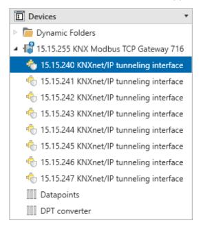
To change the individual addresses, select the corresponding entry in the list and enter the desired address in the text field under "Properties – Settings". If the frame of the text field changes its colour to red after entry, this indicates that the address entered is already being used. The changes are only applied in the device after download.
